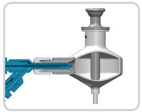
Cross section drawing of the Savillex PFA CSC with C-Flow nebulizer fitted. Nebulizer port insert eliminates dead space.
